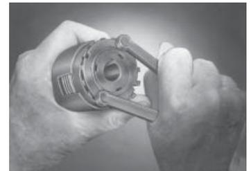
Carlyle Johnson Maxitorq® steel on bronze friction discs are considerably more predictable in dynamic and static torque properties than more commonly used fiber discs. They also last longer. Carlyle Johnson Maxitorq® coil springs maintain torque levels longer than Belleville type springs and eliminate frequent torque adjustment.
