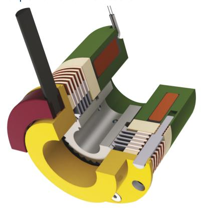
MAXITORQ® Model HBB brakes are a low cost solution when moderate torque is required in an extremely small package. The HBB brake is released when power is applied to the brake coil. When power to the brake is removed, braking torque is applied.
